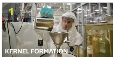
The feedstock is formed into high-density spherical fuel kernels tailored to customer specifications
