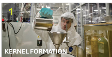
1 KERNEL FORMATION The feedstock is formed into high-density spherical fuel kernels tailored to customer specifications
